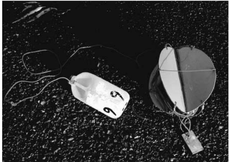
**Figure 1** A current measuring device (CMD) or drogue, which was used for tracking a water mass to determine the spatial distribution of paramoebae in the water column.
